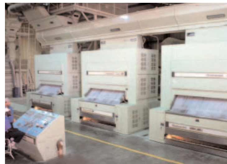
A gin typical can produce about 12 bales per hour, while some of today's "super" gins turn out as many as 60 bales per hour.
