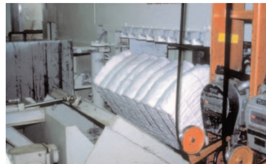
Lint from cotton is compressed into 500-pound bales.
